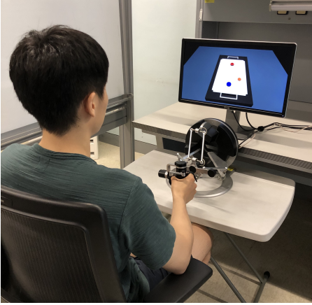
Figure 5: Experimental setup of our user study. A participant performs a virtual air hockey task with a haptic device.
